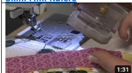
The Stitch in the Ditch Binding Foot as a 1/4" Piecing Foot
